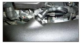
17. Connect the CCV tube to the quick connect fitting installed into the K&N<sup>®</sup> intake tube.
