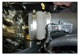
12. Install the provided hump coupler onto the air filter housing and secure with the provided hose clamp.
