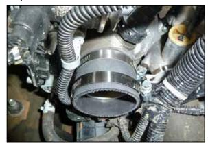
13. Install the provided straight coupler onto the turbo inlet and secure with the provided hose clamp.
