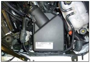
10. Remove the upper air filter housing and remove the factory air filter.
