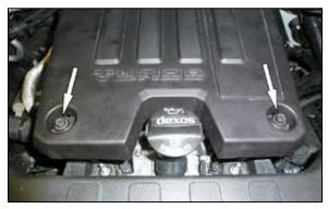
6. Remove the two bolts that secure the engine cover to the engine and then remove the cover from the vehicle. These bolts will be reused in a later step. 8. Using the factory bolts and the nuts provided, secure the two provided "Z" brackets to the engine cover as shown.
